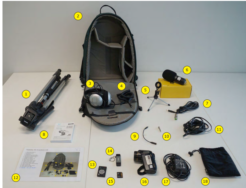
Figure 9.12: The portable usability kit used at Graz University of Technology. The inventory shows all of the components of the kit.
