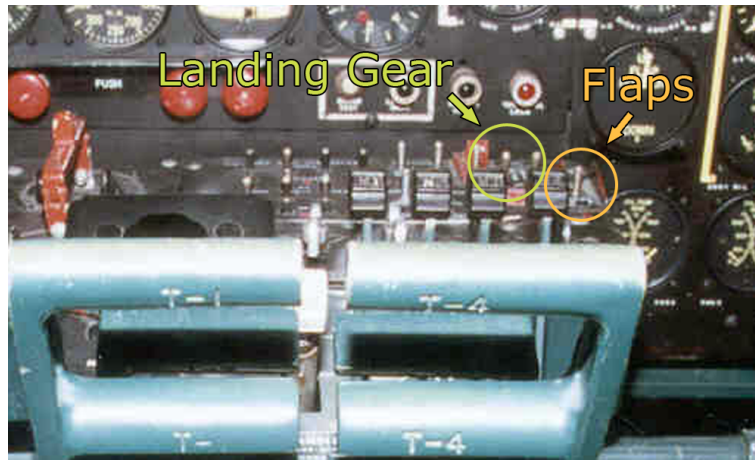
Figure 2.34: Close-up of the cockpit control knobs of a B17G Flying Fortress. The landing gear and flaps control knobs are identical and are very close to one another. [From USAF [2006], image believed to be in the public domain.]
