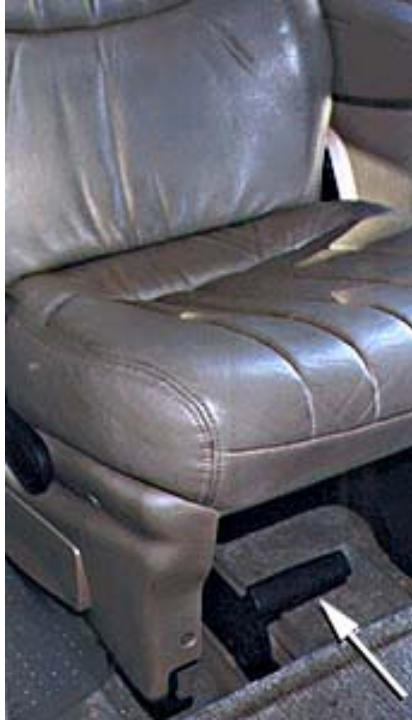
Figure 2.15: The lever beneath this mini-van seat does not work as expected. Instead of allowing the seat to slide backward or forward, pulling the lever detaches the seat from the floor to make room for cargo! [Photograph courtesy of Baddesigns.Com [Darnell 2010].]
