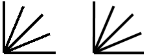
Figure 9.11: The lines on the left illustrate aliasing, they have jaggy steps along the edges. On the right, the black lines are antialiased against a white background by adding intermediate (grey shade) pixels to fade gently from foreground to background.
