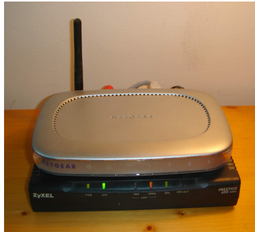
Figure 6.2: The bottom device is the broadband (xDSL) modem provided by the internet provider (inode). The top device is a wireless router providing wifi throughout the flat.
