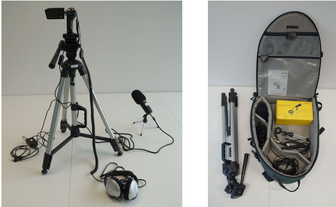
Figure 9.13: The portable usability kit used at Graz University of Technology. On the left, the kit has been set up ready for use. On the right, the kit packed up.
