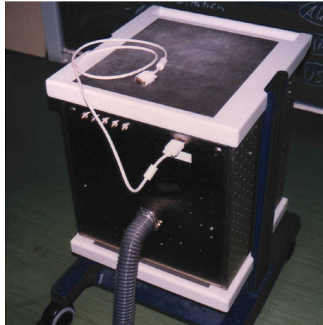
Figure 2.5: The audiovisual trolley in lecture theatre HS EDV has input connectors at the rear. Unfortunately, unscrewing the external connector causes the internal connector to fall with a clunk somewhere inside the trolley!
