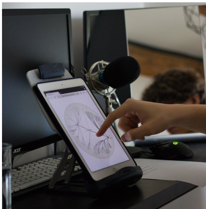
Figure 9.5: Testing on a tablet using a book stand. An external camera, mirror, and table microphone are being used, in addition to screen video capture and audio capture on the tablet. [Image used with kind permission of Chris Oser.]
