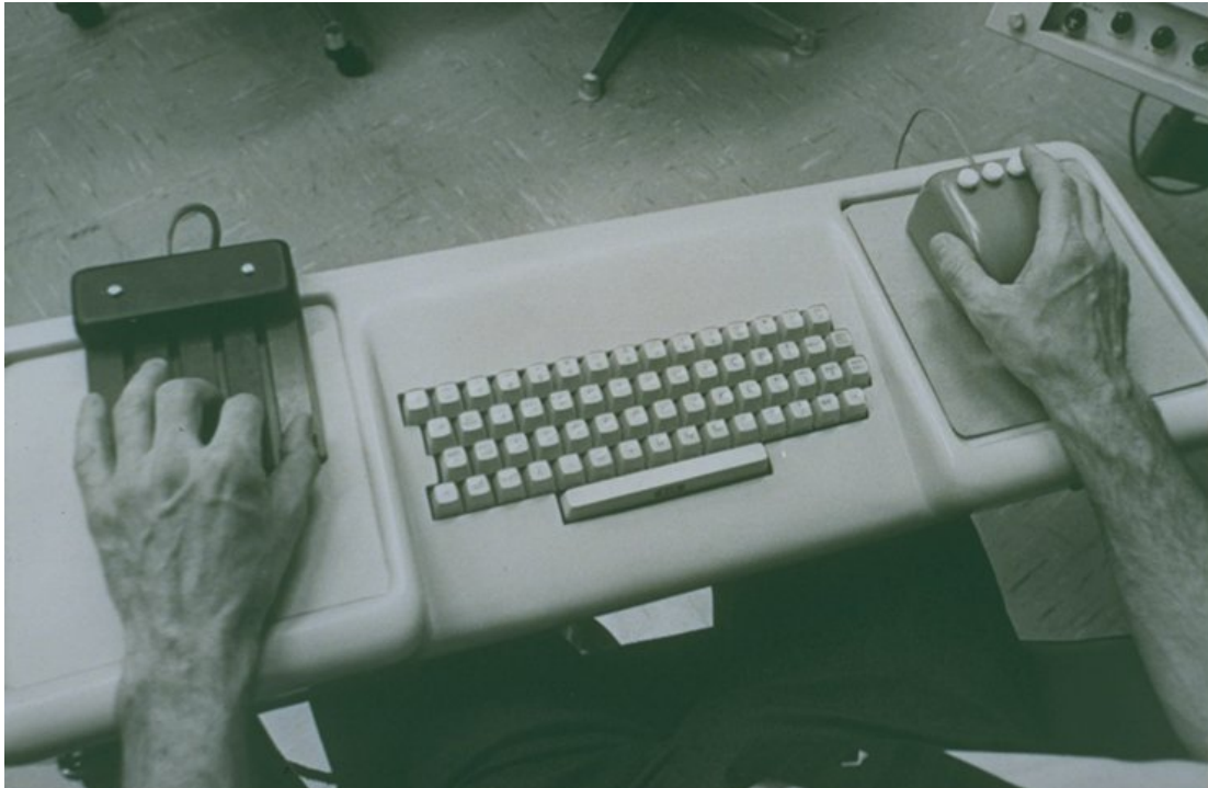
Figure 13.7: The NLS Mobile Keyboard used by Doug Engelbart in the famous 1968 live demo. Mounted across a office chair on wheels. Five-chord keyset on the right, keyboard in the middle, and mouse to the right. [ Image used courtesy of SRI International, Menlo Park, California. ]
