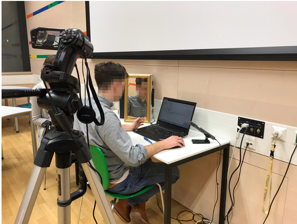
Figure 9.4: Simple usability test setup in 2019. An external camera, mirror, and table microphone are being used, in addition to screen video capture and webcam capture on the laptop. [Image used with kind permission of Angelika Droisner and Ana Korotaj.]
