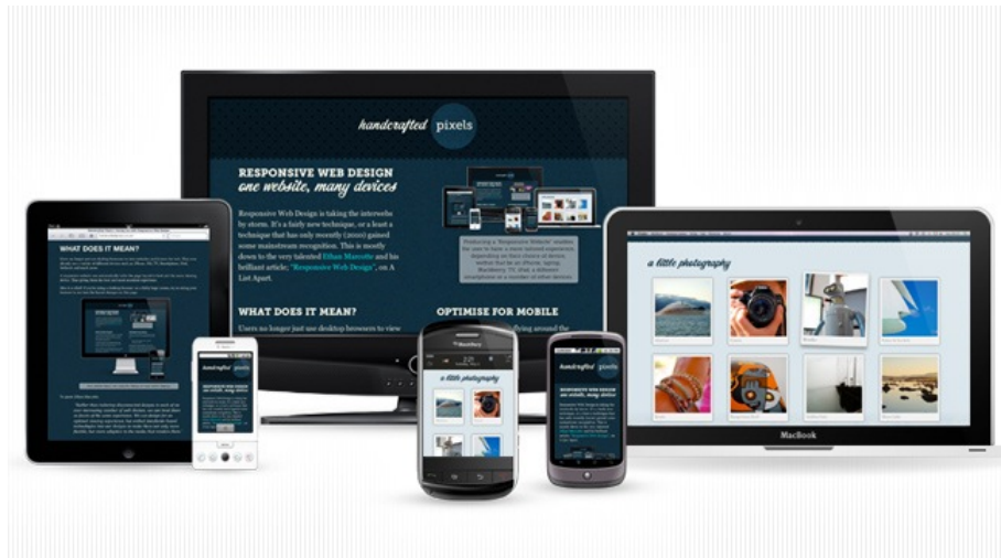
Figure 2.1: Displaying a website on various devices in different resolutions using media queries
