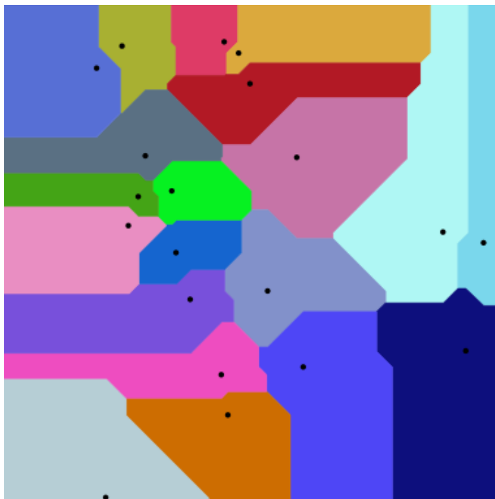
Figure 2.2: A Voronoi Diagram using the manhattan distance as distance function [Diagram taken from Wikipedia]
