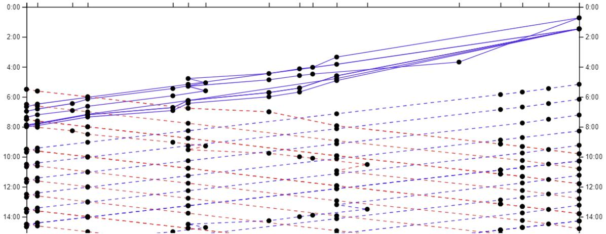
**Figure 8.1:** Zig-zag lines caused by non-linear train stops. [Screenshot made by Elliot Koh using String Charter.]
